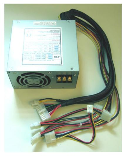
320W DC ATX P4 Power Supply (9-18VDC)
